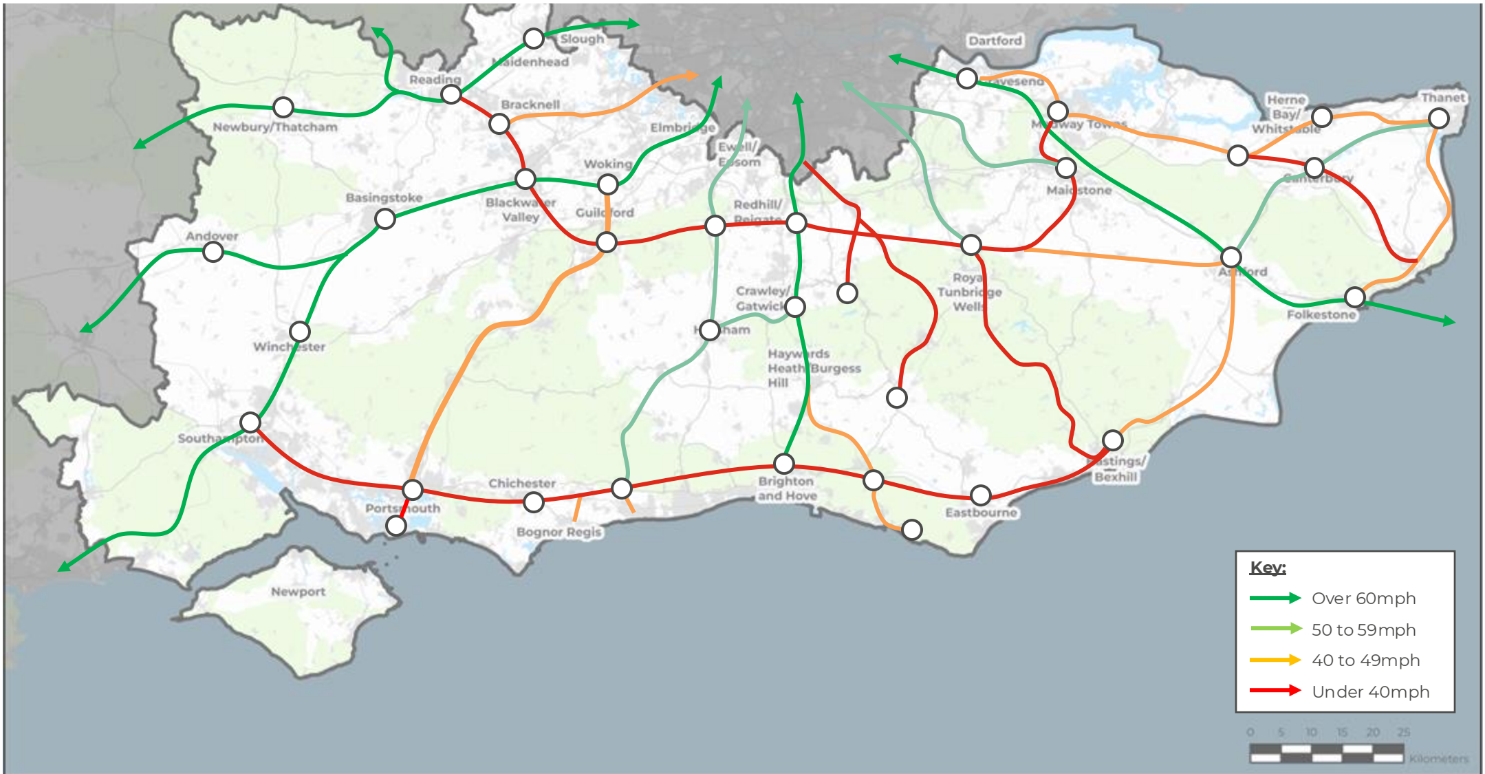
Figure 1.23: Railway connectivity in the TfSE area (average rail speeds on corridors between major centres)
